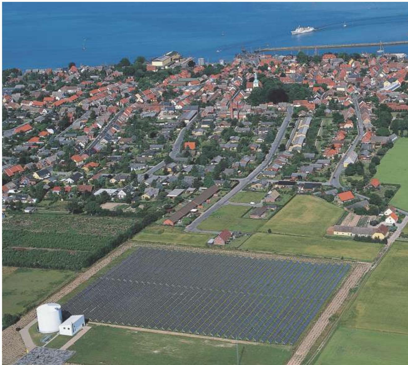
2002 - To increase the solar fraction for the town's district heating system, the solar collector area is raised to 18,000 m<sup>2</sup>.
