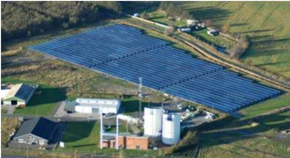
Top - 8,000 m<sup>2</sup> of ground-mounted solar collectors help to heat the small town of Strandby, Jutland.
